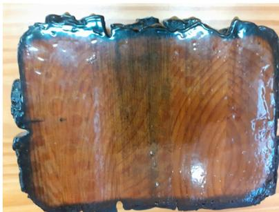
After 30 minutes in furnace charring depth showed 18mm = 30 mins x .6mm per minute
