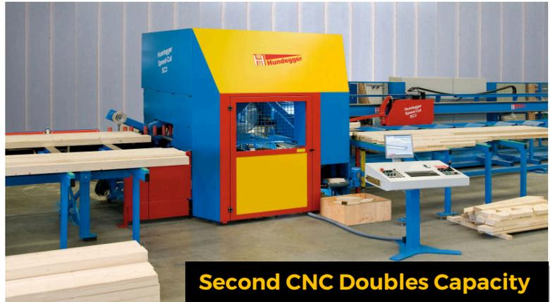
The fully automated Hundegger Speed-Cut SC-3 (purchased in 2018) greatly increases our capacity in processing smaller section linear product, allowing us to focus our Weinmann WMP240 on the more complex or larger-section projects. TimberLab is the only NZ Glulam fabricator at this time to operate 5-axis CNC technology.
