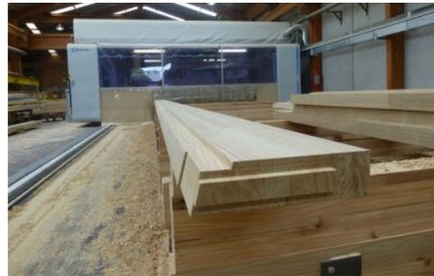
The WMP240 processes solid timber elements 35 m long - 4 m wide and 450 mm thick.
