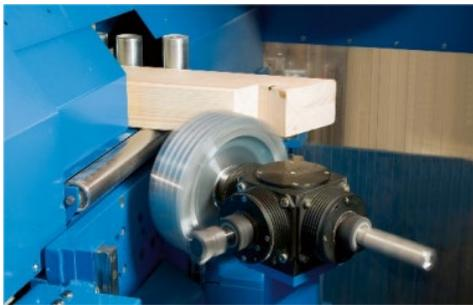
The SC-3 processes solid timber elements 200 mm x 450 mm x up to 8 m.
